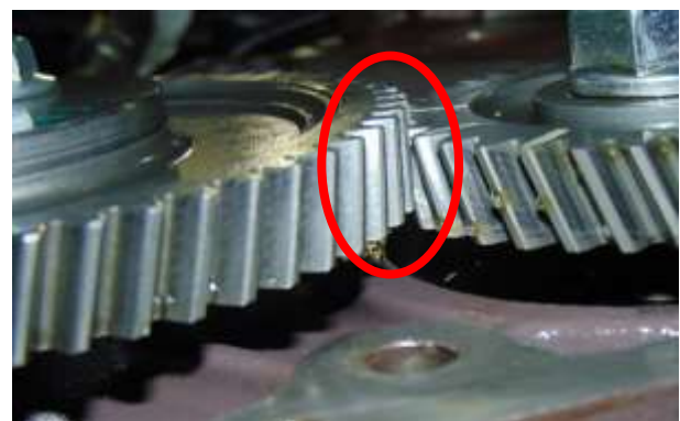
Fig:11 Baseline idler gear position on engine
