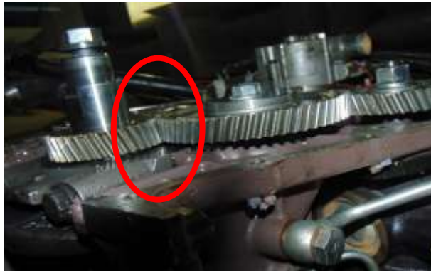
Fig:12 Modified idler gear position on engine
