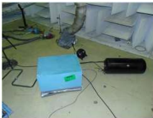
Fig: 9 Compressor Brake System dryer with Acoustic covered
