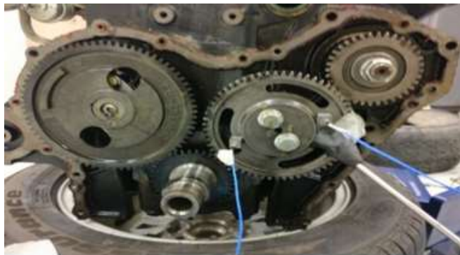
Fig:5 Idle gear that is removed when compressor is driven by belt change in drive makes unwanted noise get reduced
