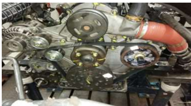
Fig:6 Compressor is driven by belt drive
